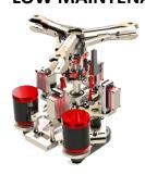
Velos UAV is an extremely low maintenance helicopter. The simplicity of the twin electric power train requires replacing only a few ball bearings and two belts every about 80-100 hours but that can easily verified with a simple inspection and can be performed in 15 minutes! Nothing like the gas powered UAVs.
