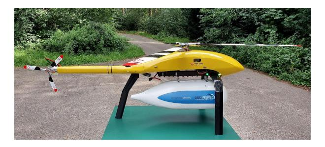
The Velos UAV is a professional UAV helicopter designed in way that it can be easily adapted in a variety of different applications. The unique payload rail system provides plenty of flexibility and free space thus allowing almost any possible payload to be mounted on the helicopter in a fast, easy and reliable way. Furthermore, it is very easy to switch between different equipment, e.g. remove a gimbal and add a thermal camera or a LIDAR in few minutes.
